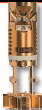
Ultra-compact TESLA JT SPM head. The use of non-magnetic material allows for the operation at virtually any magnetic field.
